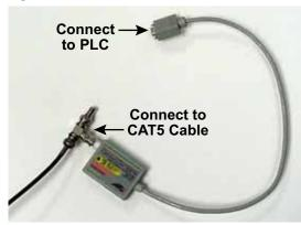
Figure 1-2: Coax Cable on Touch Screen
